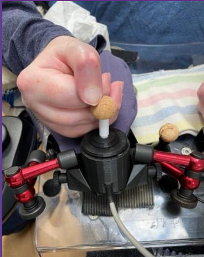
Smaller HSB2 with no optional switches used for mouse control whilst the user is in his wheelchair
